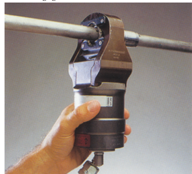
Position PYPELOK® tooling around fitting assembly and pressurize.
